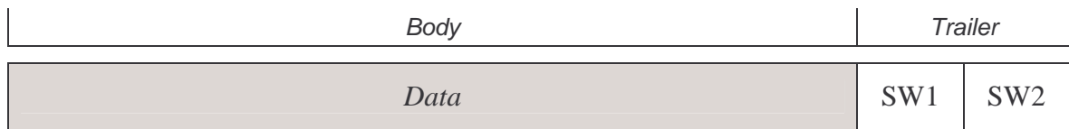
Figure 7.2: ISO 7816-4 Response APDU structure
